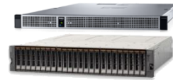
Dell C4130 with 4x NVIDIA Tesla K80 512 GB RAM + iSCSI JBOD (20TB)
